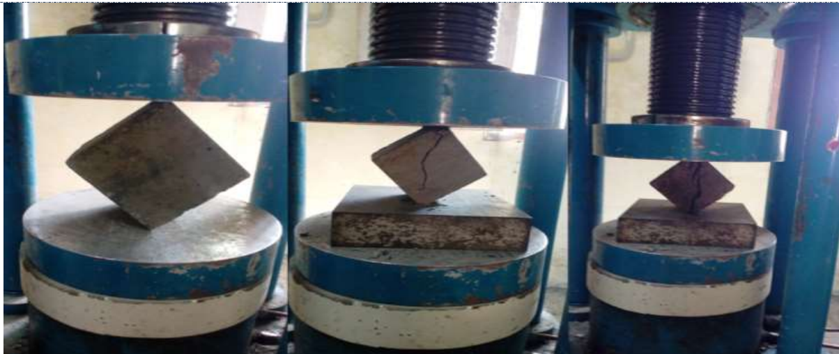
Fig.4: Tensile Strength Test Setup
